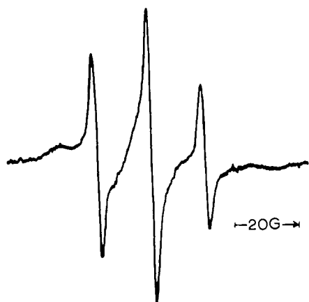
FIGURE 2: Electron spin resonance spectrum of ATCase labeled with 4- \alpha -iodoacetamido-2,2,6,6-tetramethylpiperidine- N -oxyl, recorded at 23° in pH 7.0, 0.04 M phosphate buffer.
